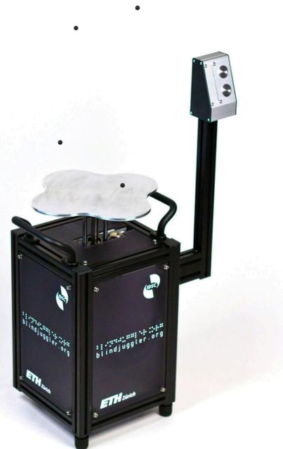
Fig. 1. The Blind Juggler bouncing four balls on the Cloverleaf paddle. The user interface features two buttons to control the juggling machine.
