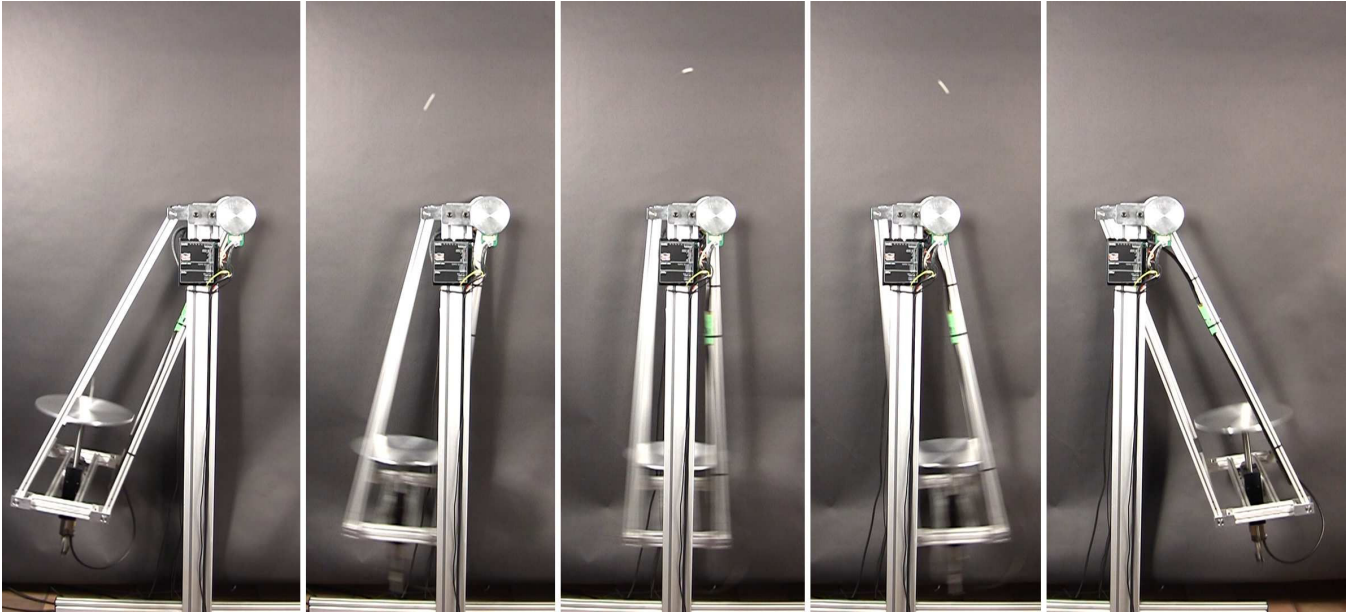
Fig. 2. The Pendulum Juggler juggling at an amplitude of 25^\circ . The round structures at the top are brushless motors controlling the pendulum motion.
