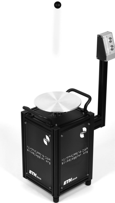
Fig. 1. The Blind Juggler bouncing a superball. The user interface features two buttons to control the juggling height.
